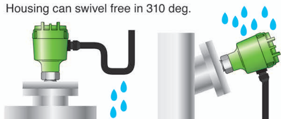
Prevent water intrusion by warping wiring cable
